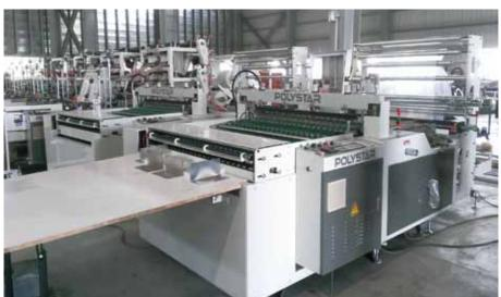
The side sealing bag making machine is available for producing different types of side sealed plastic bags. The multi-functional side sealing bag making machine in total can produce 15 different types of side sealing plastic bags. Clothes packaging bags, bakery bags, stationary packaging
